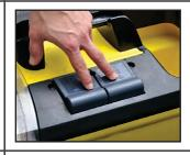
Press both buttons on the top of the carpet cleaning machine to switch on the spray and the suction.
